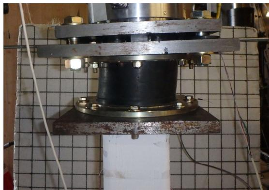
**Figure 2-6:** Pure rotation test at +0.02 rad of top rotation
