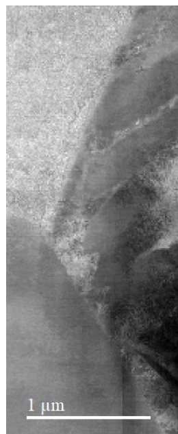
Figure 62: TEM image of the ferrite/austenite interface.
