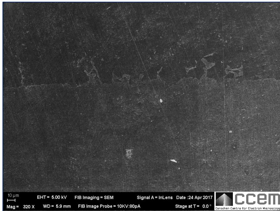
Figure 31: SEM image of ferrite precipitation in the Fe-1.5Mn-1.3Si-.66C sample.
