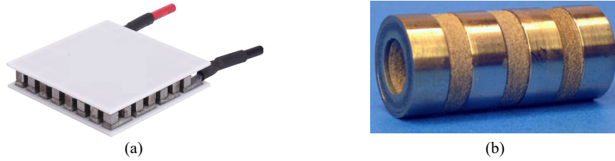
Figure 3.2: (a) off-the-shelf flat TEG module (b) cylindrical TEG module concept [63].
