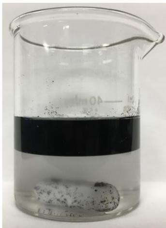
Figure 4.5: Extraction of MWCNT from the aqueous phase (bottom) to the 1-butanol phase (top).
