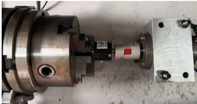
Figure 6.3 Static characterization test setup: left to right: rotor position holder; static torque sensor; coupling; electric machine.
