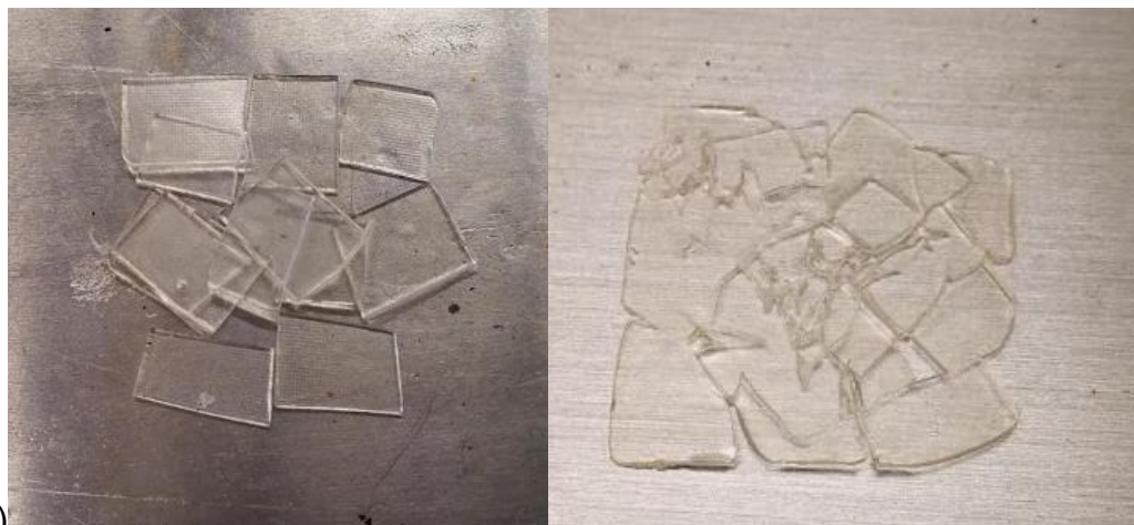
Figure S5.6. Reprocessing of (a) taPEVA and (b) tsPEVA under hot press at 160 °C for 20 min.
