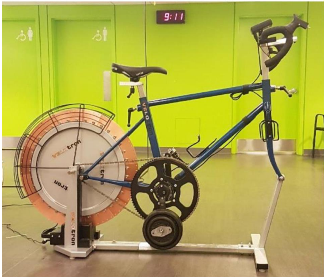
Figure 4; Single-leg cycle ergometer set-up. Velotron, RacerMate cycle ergometer specially adapted with 11.4kg counterweight.
