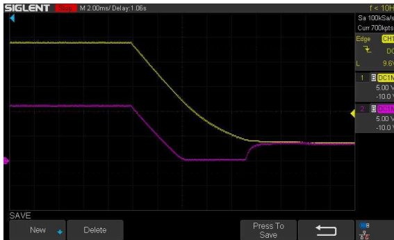
Figure 5.18 Power off a normal channel
