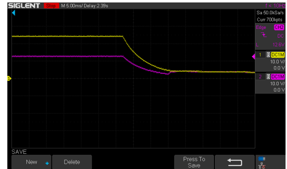
Figure 5.19 Power off a saturated channel
