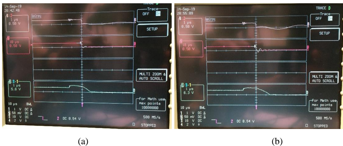
Figure 5.23 OCP with the crowbar circuits
