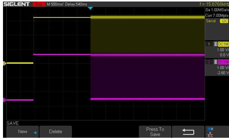
Figure 5.30 A delay of 2 s before the start of I2C communication
