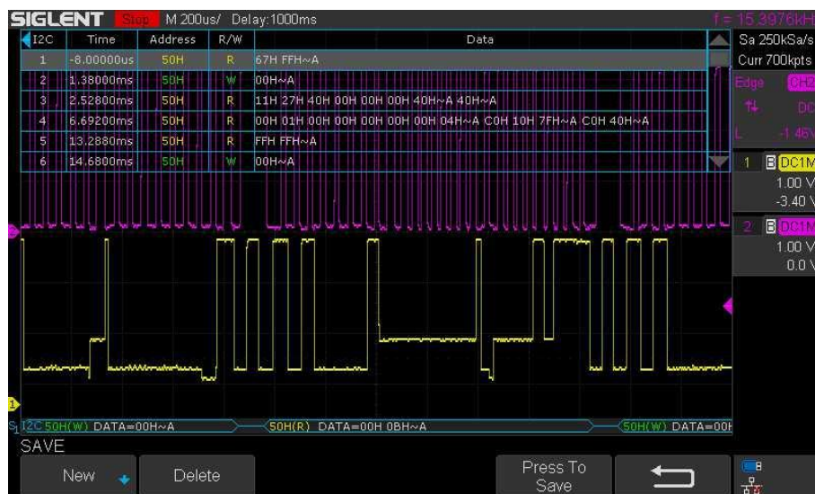
Figure 5.37 Error in I2C due to the pull-up resistors
