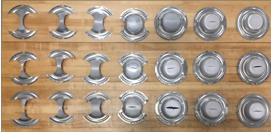
Figure 5.2.5 Deformed Marciniak test samples; sample geometry from uniaxial tension to balanced biaxial tension (left to right) and 300°C to 400°C (top to bottom)
