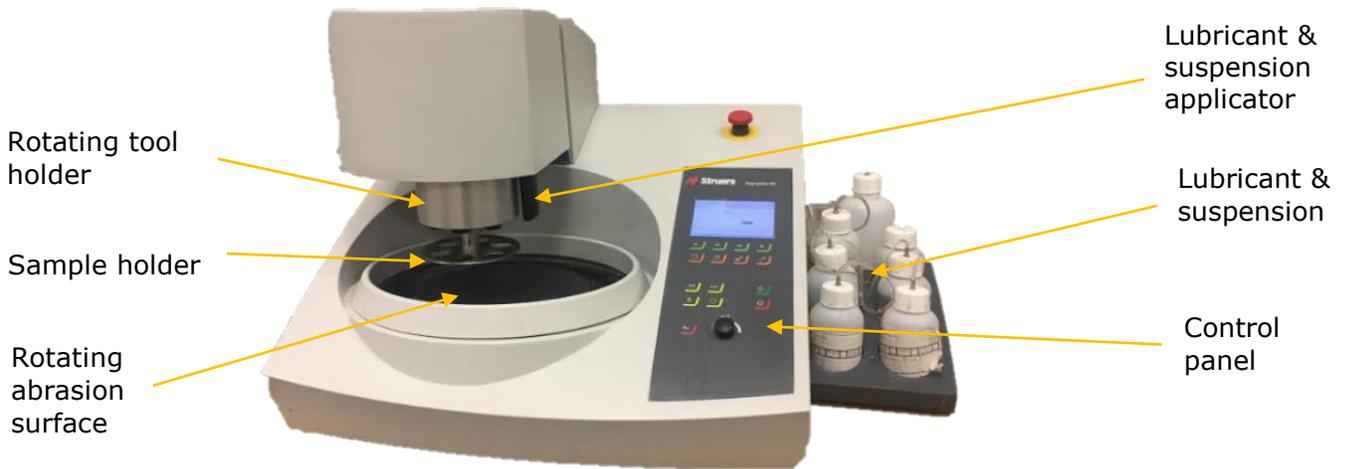
Figure 3.6.3 STRUERS Tegramin-25 semi-automatic polishing machine
