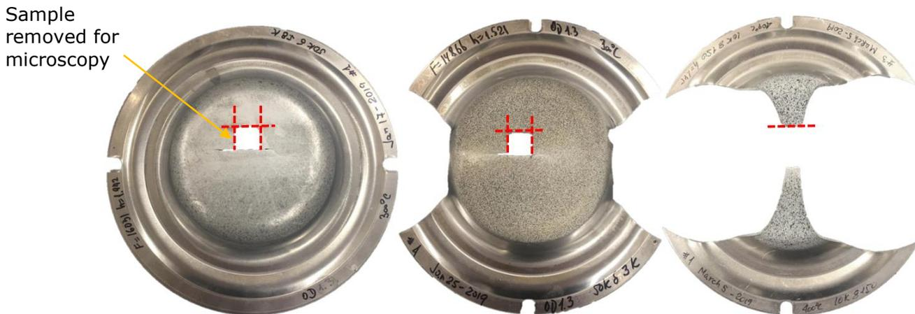
Figure 3.6.1 Fracture surfaces cut from formed Marciniak test for fractography
