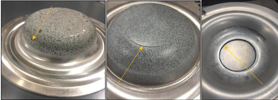
*Figure 3.4.4 Specimen fracture characteristics, (a) edge fracture due to small punch radius, and (b, c) fracture due to stress concentration around carrier hole reaching punch radius apex*
