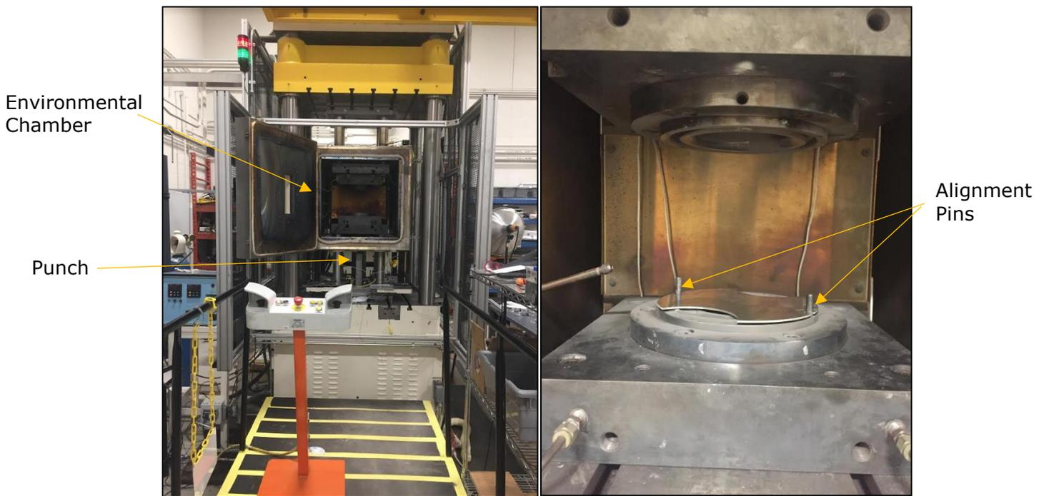
*Figure 3.4.1 MACRODYNE press and forming setup with high temperature capability*
