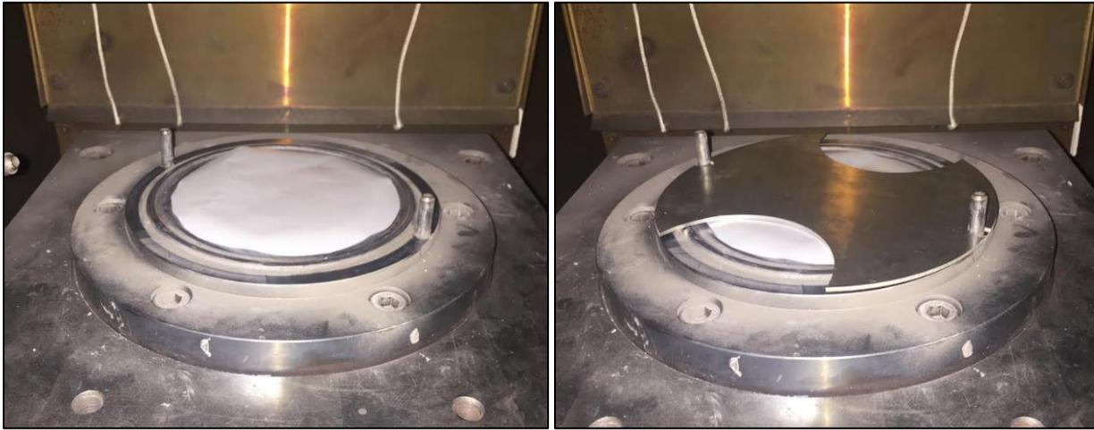
*Figure 3.4.6 Teflon lubricant and blank placement for high temperature Marciniak test with alignment pins*
