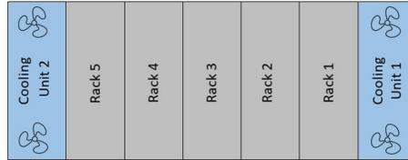
Figure 6: Location of fans in cooling units
