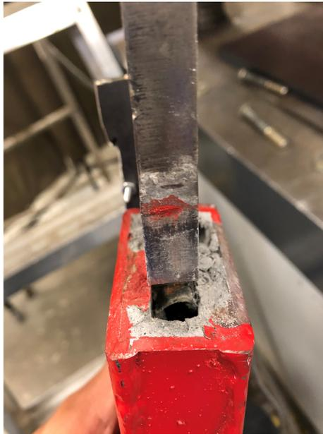
Figure 3.18: VL LONG Specimen: Yielding core after tension half-cycle
