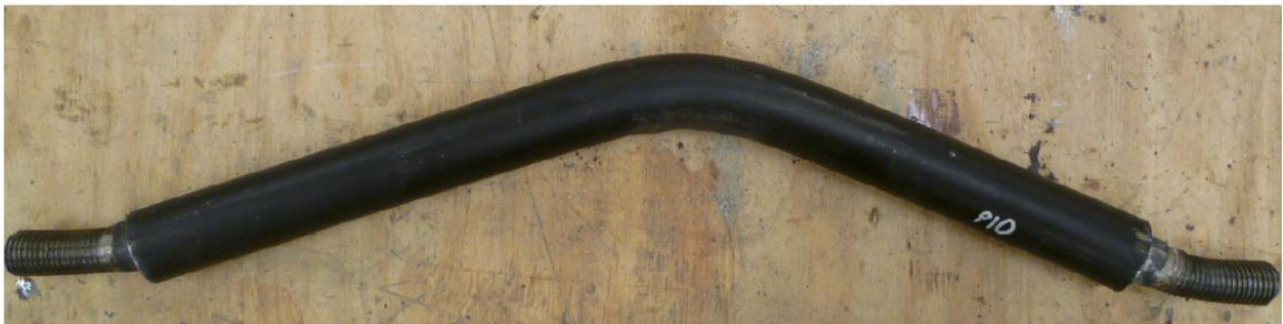
Figure 2.13: Buckling of Sarti's fuse (2016)
