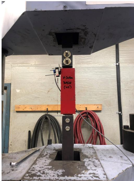
Figure 3.6: String potentiometer installation
