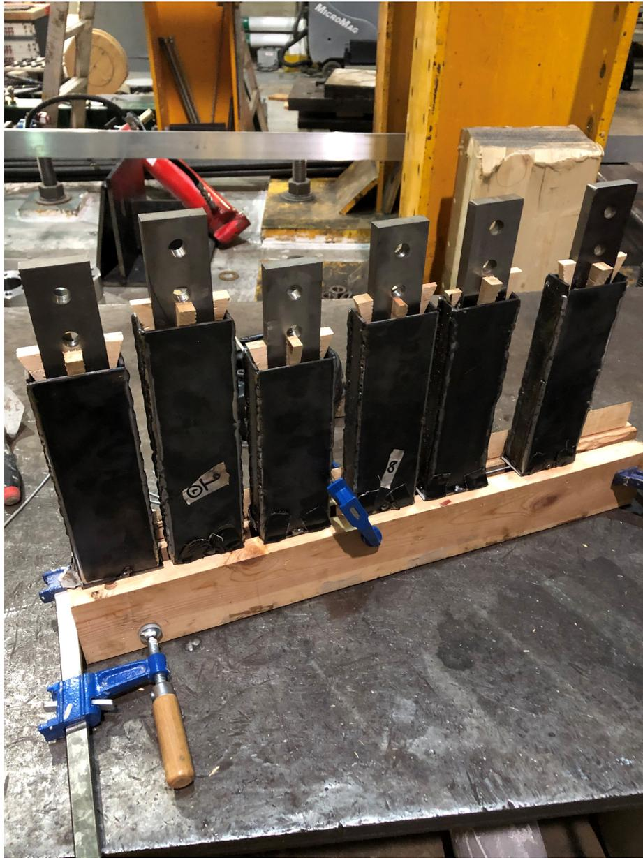
Figure 3.12: Temporary wedges used during grout pouring
