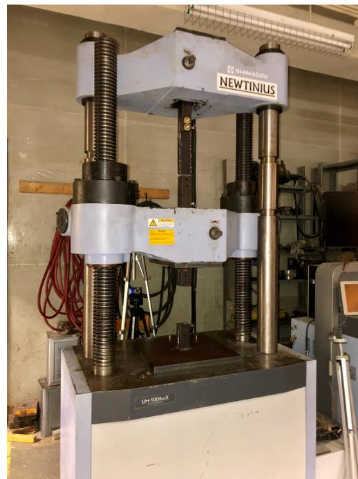
Figure 3.5: Full assembly of adapter installed into the Shimadzu
