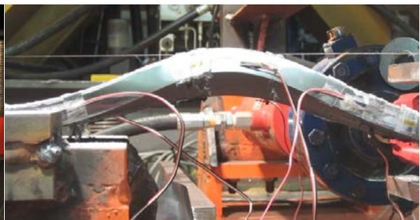
(j) Max Displacement - Side View (90 mm)
