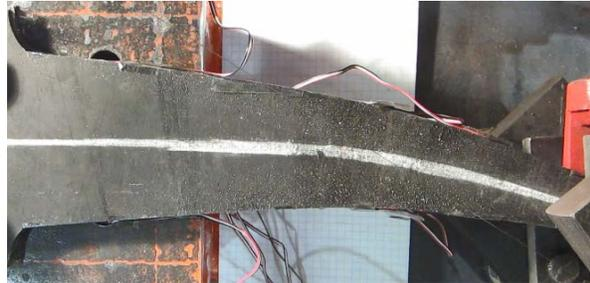
(a) Target Displacement – Top View (47 mm)
