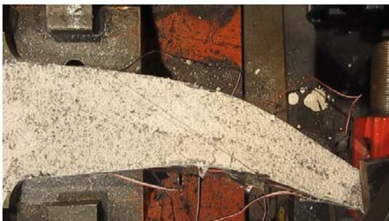
(i) Max Displacement - Top View (90 mm)
