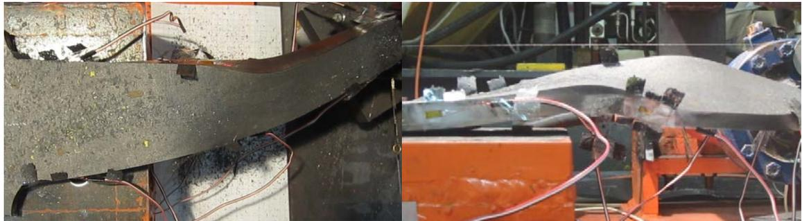
(i) Prior to Failure – Top View (4x90 mm)
