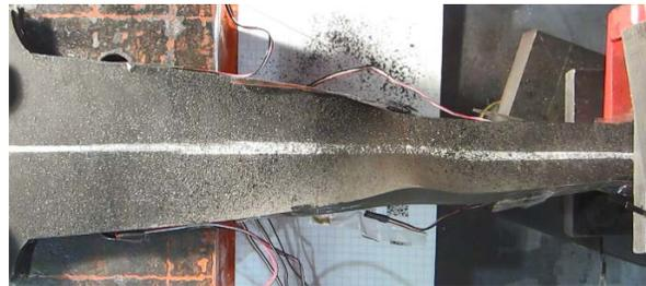
(c) Failure – Top View (2x90 mm)
