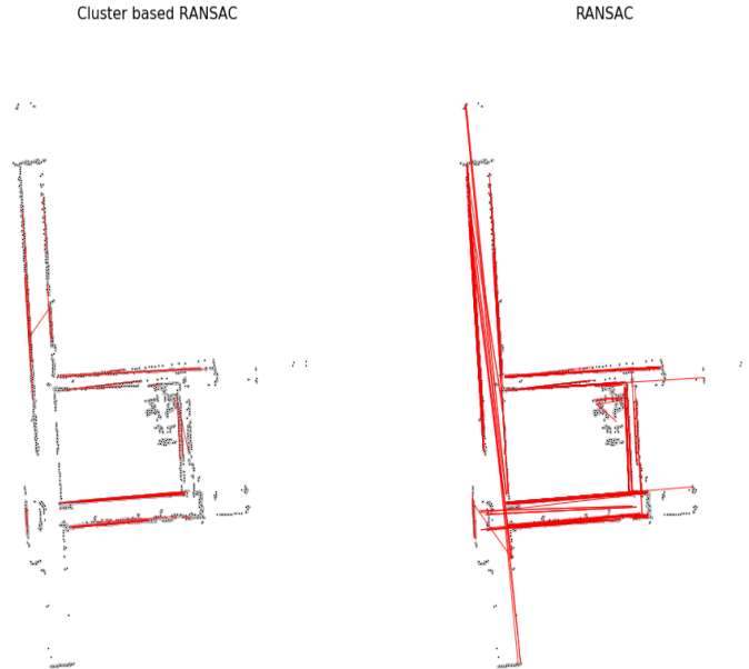
FIGURE 5.11: Walls extracted superimposed on real data, by selecting a subset of 15 scans
