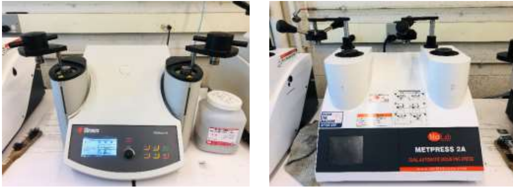
Figure 3.10 Struers CitoPress-20 and MetLab METPRESS 2A Hot Mount machine with Black Phenolic Thermosetting powder
