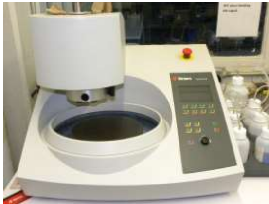
Figure 3.11 Struers Tegramin-25 Auto polisher
