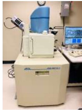
Figure 3.13 JEOL JSM-6610LV SEM device
