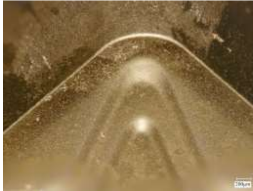
Figure 3.2 Coated Carbide insert preview Cutting edge of B0
