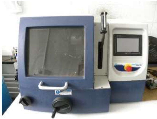
Figure 3.9 AbrasiMatic 300 Abrasive cutter
