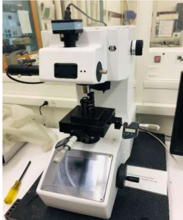
Figure 3.7 CLEMEX intelligent – CMT High Definition microhardness tester
