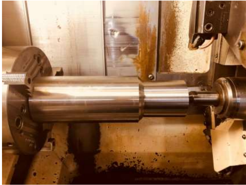
Figure 3.5 Machining set up in Boehringer three-jaw clamps, cylinder shape of AISI 1018, Coated carbide insert B0
