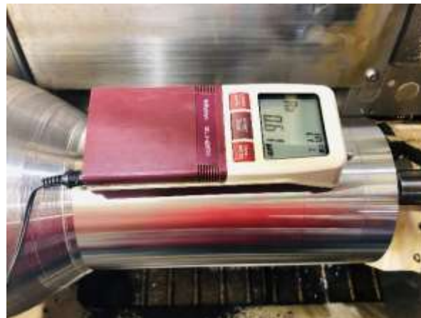
Figure 3.8 Mitutoyo SJ-201 handheld surface roughness tester, Boehringer lathe, cylinder shape of AISI 1018
