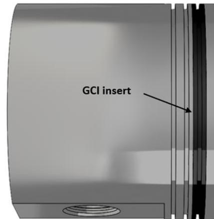
Fig. 7 AlSi-GCI Piston used for bimetal machining study [20]
