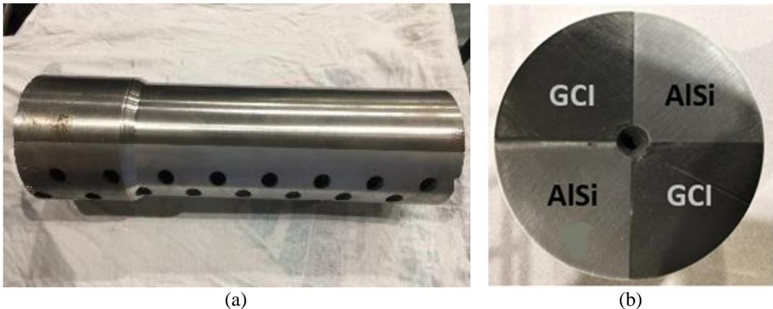
Fig. 13 Manufactured AlSi-GCI bimetal workpiece a) Front view (b) Side view
