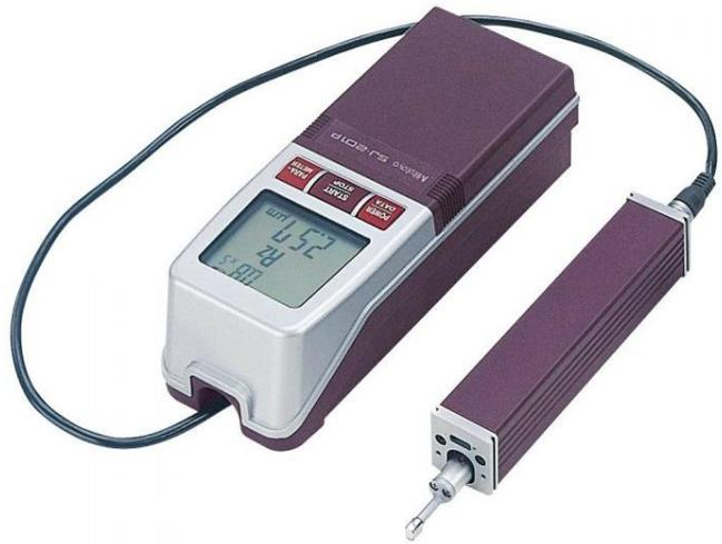
Fig. 18 Mitutoyo roughness tester sj-201
