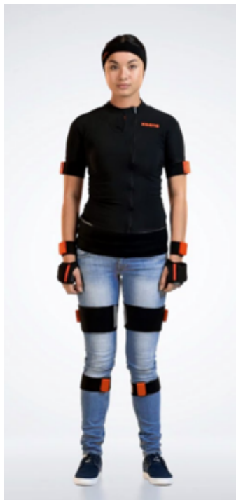
Figure 2.1: Photo of the MTw Awinda system used for collection of postural data. Note the inertial sensors that are shown in orange. Image from xsens.com.
