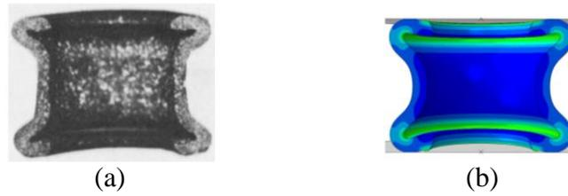
Figure 3.17: Comparison of (a) the result of experiment from a paper [Hartley et al., 1981] with (b) the result of simulation for the verification of procedure in ABAQUS.
