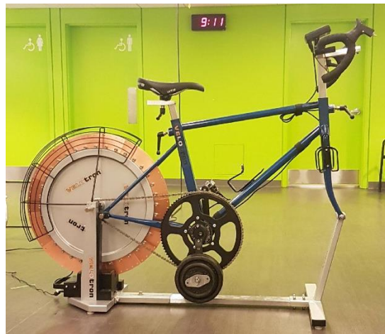
Figure 1. A cycle ergometer adapted for counterweighted single-leg cycling. An 11.4 kg counterweight is placed on the crank arm of the non-active limb.
