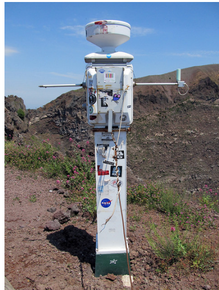
Figure 1.4. Seismic monitoring devices such as the one pictured here provide continuous data about subsurface vibrations at Mount Vesuvius (Chouet, 1996).
