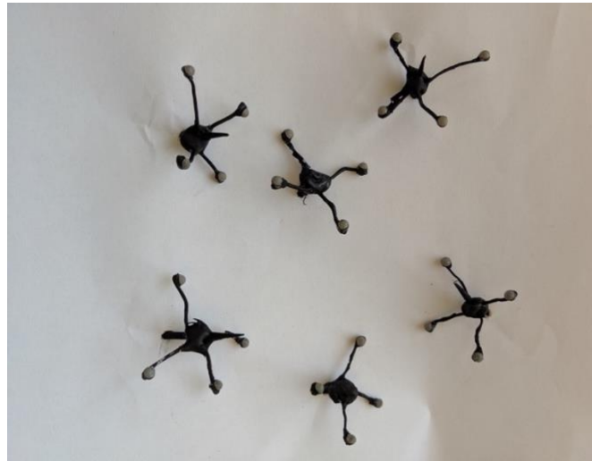
Figure 3.4: Marker Clusters Used for Tracking Motion of the Fragments.
