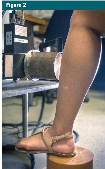
Figure 2: Tibial gadolinium measurement was performed with a 180° set-up geometry, in which the subject's leg was placed directly in front of the ^{109}\text{Cd} source.
