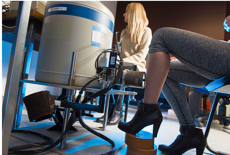
Figure 2.6: The setup for a human tibial measurement of Gd in bone using an XRF detection system. Photo by: Paulina Kowalczyk.
