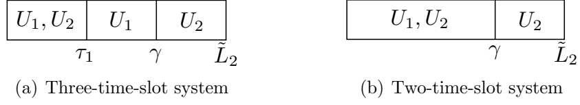
Figure 2.13: In the three-time-slot system there is one time slot (the second) in which user 1 is the only user transmitting. In the two-time-slot system user 1 completes its transmission in the first time slot and only user 2 has a slot in which it transmits alone.
