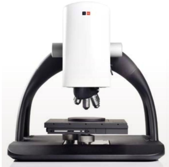
Figure 3. 8 SENSOFAR® METROLOGY S Neox 3D Optical Profiler located at National Research Council (NRC), London, ON [81]
