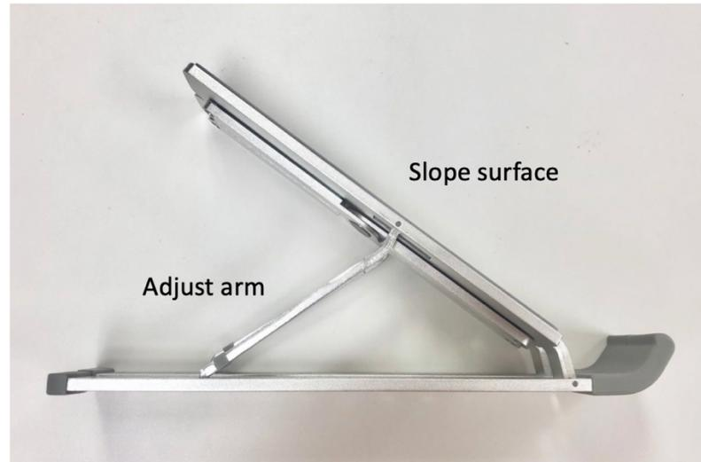
Figure 3. 12 Device used to measure the sliding angle
