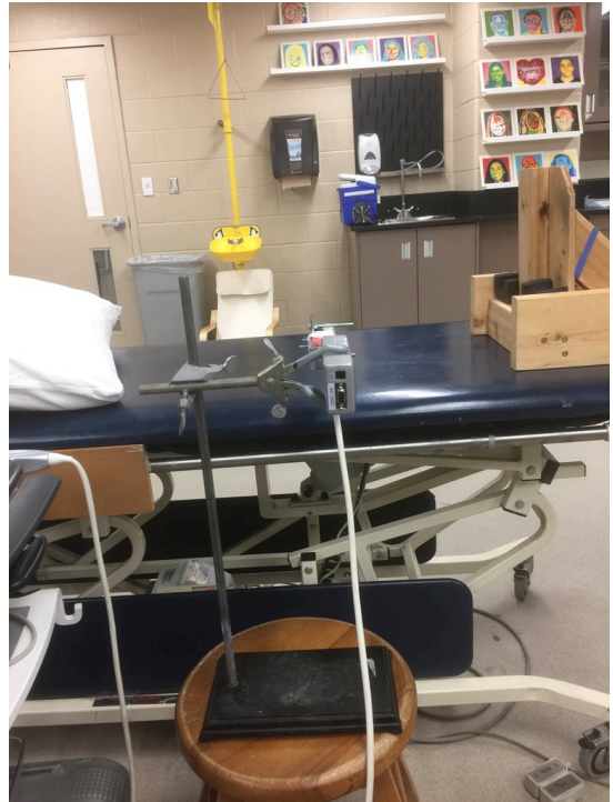
Supplementary Figure 2. Panel A: Lateral view of the mount used to assess pressure during ultrasonography. Panel B: Frontal view of the mount used to assess pressure during ultrasonography including the apparatus used to elevate the participant's leg from the bed.
