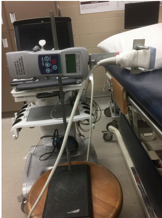
Supplementary Figure 2. Panel A: Lateral view of the mount used to assess pressure during ultrasonography. Panel B: Frontal view of the mount used to assess pressure during ultrasonography including the apparatus used to elevate the participant's leg from the bed.
