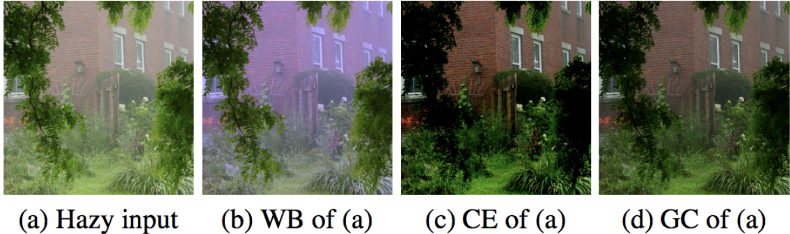
Figure 2.6: Input of GFN. WB, CE and GC denote White Balance, Contrast Enhancement and Gamma Correction respectively. (Image originally used in Ren et al. (2018))
