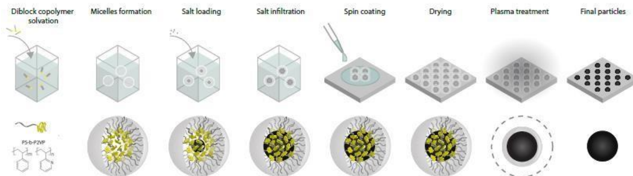
Figure 2.18. Preparation of nanoparticles using the diblock copolymer reverse micelles(92).
