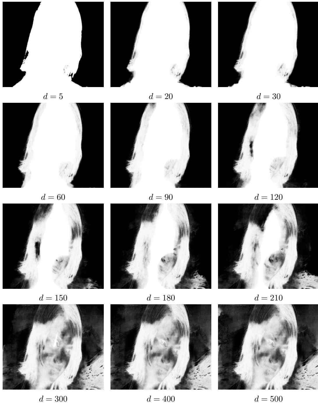
Figure 5.5: Trimap dilation result that represent the results trend with respect to dilation parameter d variation.
