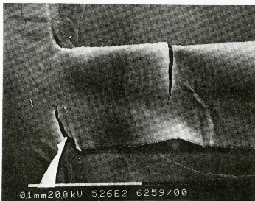
**Figure 4.23** SEM image of a 100 micron wide wire exposed to a single laser pulse at a fluence of  $121 \text{ mJ/cm}^2$ . The fluence was large enough to damage the wire.
