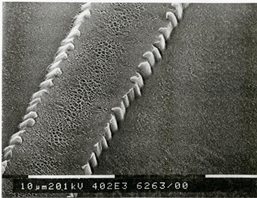
**Figure 4.22c** Magnification of Figure 4.22a showing the region where the aluminum wire has inadvertently been lifted up in preparation for SEM, thereby revealing the underlying polyimide.
