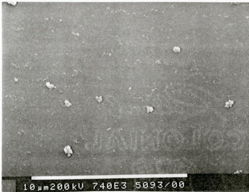
**Figure 4.17b** SEM image of the silicon surface following removal of the multilayer.
