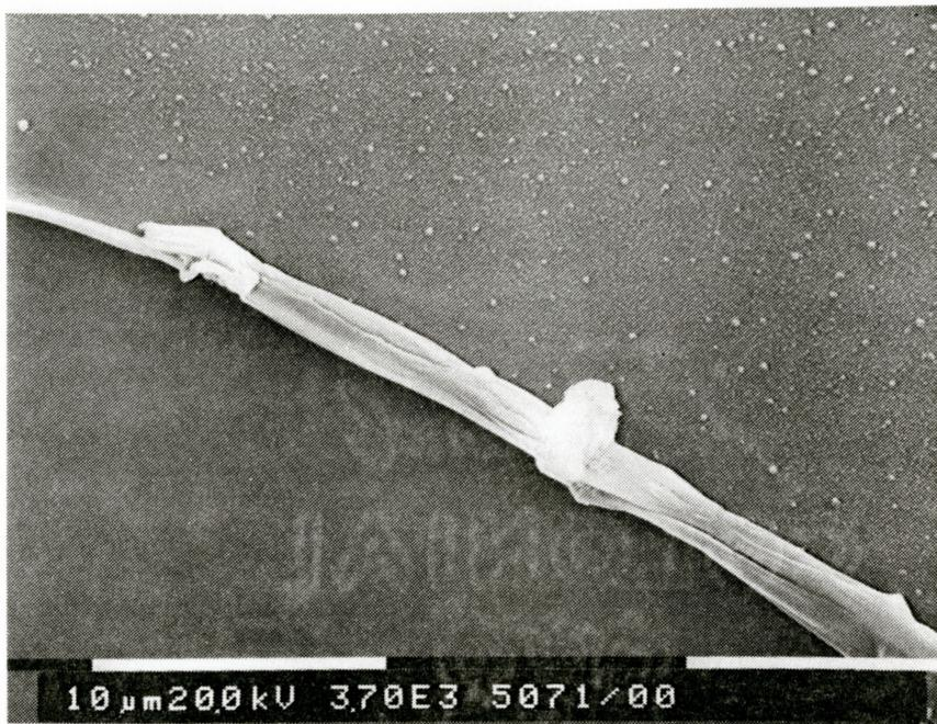
**Figure 4.9c** SEM image showing the edge quality of the hole in Figure 4.9a.
