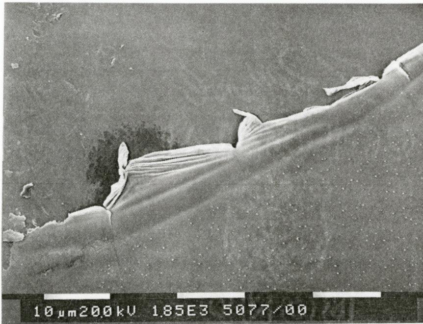
**Figure 4.10b** SEM image showing the edge quality of the hole in Figure 4.10a.
