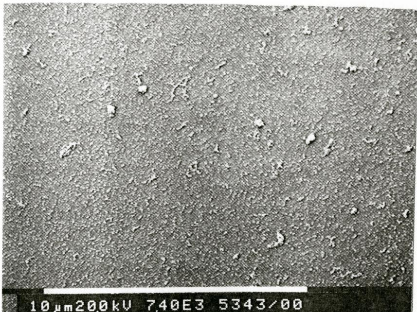
**Figure 4.4b** SEM image of the bottom of a hole created by four pulses at a fluence of  $187 \text{ mJ/cm}^2$ .
