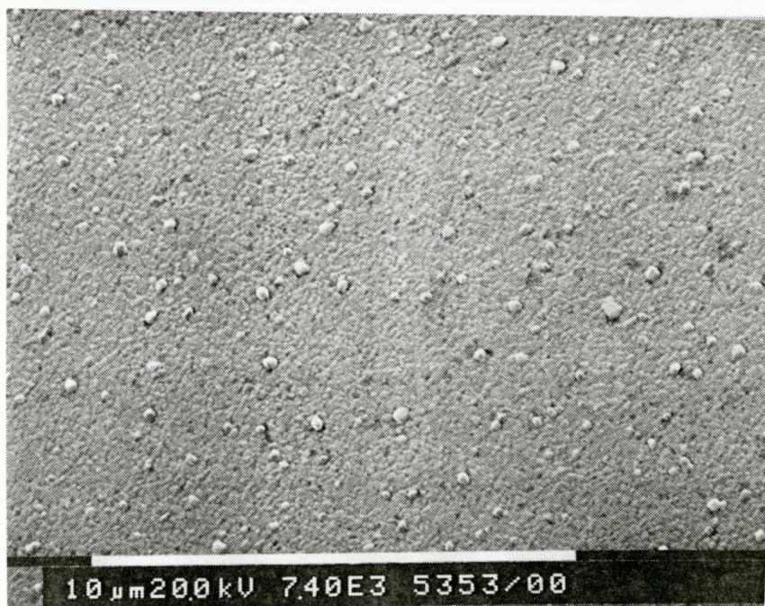
**Figure 4.15d** SEM image showing the surface of a section of the aluminum layer which has not been exposed to laser light.
