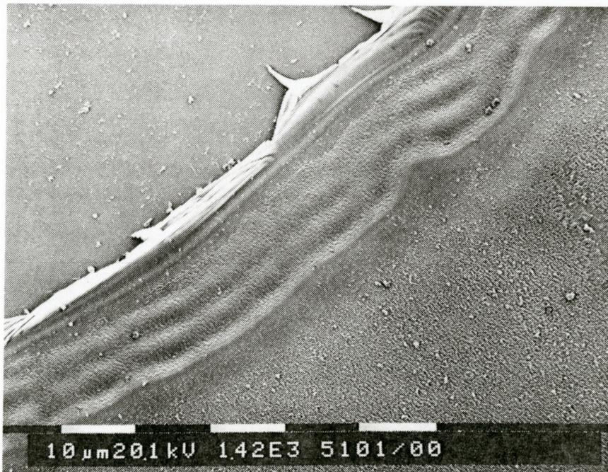
**Figure 4.16d** SEM image showing the edge quality of the hole in Figure 4.16a.
