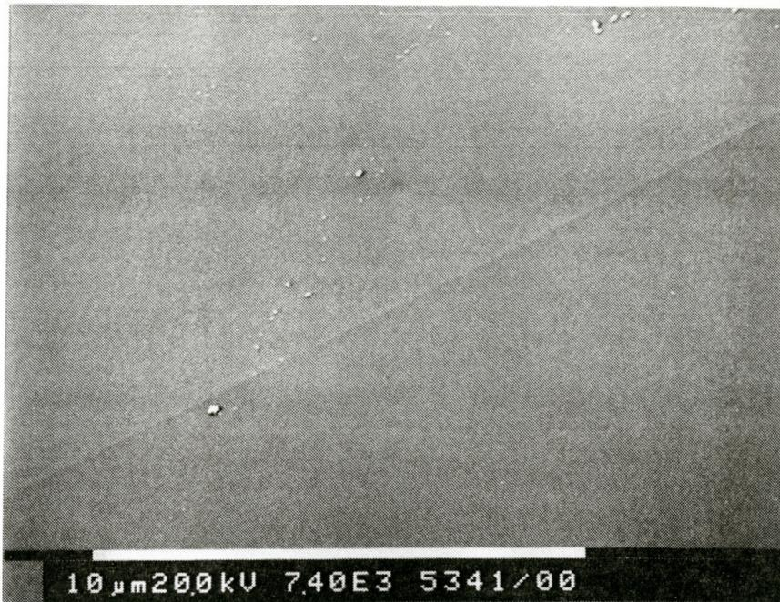
**Figure 4.4a** SEM image of the polyimide surface prior to irradiation.
