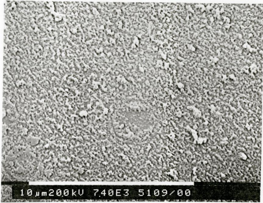
**Figure 4.15e** SEM image of debris surrounding the hole shown in Figure 4.15a.
