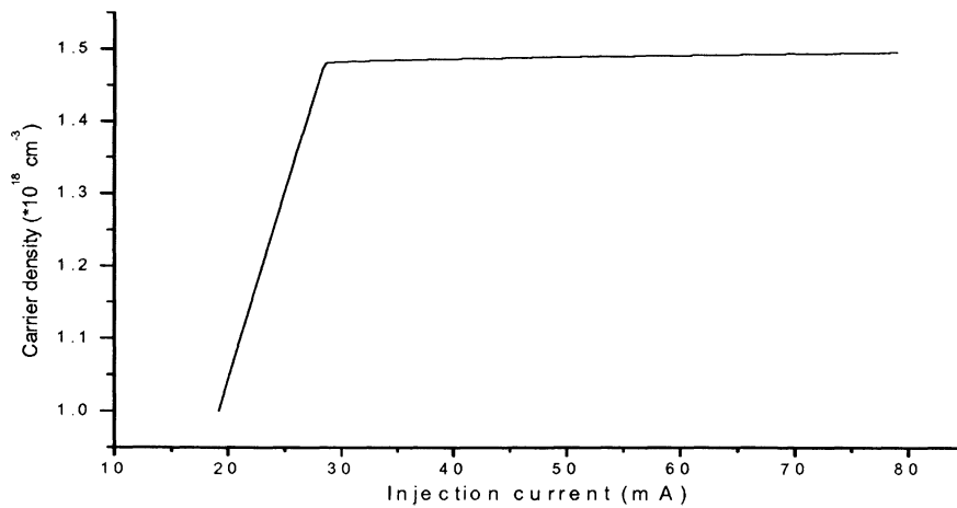
Figure 5-8 Carrier density V.S. injection current for multi-mode steady state
