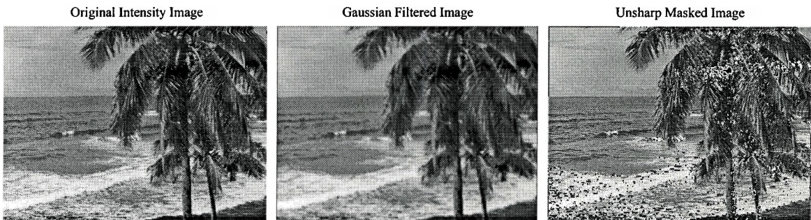
Figure 2.5 Gaussian low-pass filtering ( \sigma^2 = 0.49 ) with 3 x 3 convolution mask to smooth an 8-bit intensity image
