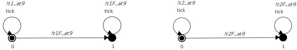
Figure 15.39: Sensor 9 and Train 1 with Figure 15.40: Sensors 9 and Train 2 with Permanent Faults
