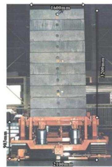
**Figure 1-2:** 3D isolation system including multi-stage rubber bearing and coil spring and damper [4]
