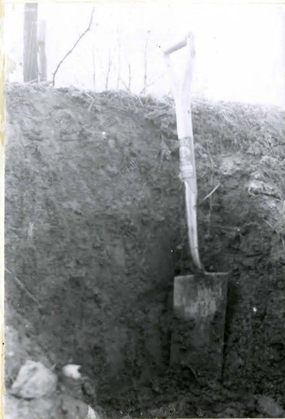
Photo 9. A soil profile in the Napanee Clay Loam. AI - A dark brown humus layer - 6" thick. A2 - Lighter in colour, yellowish, slightly leached layer - 14" thick. B - Well developed compacted, heavy textured layer, dark brown to reddish in colour.
