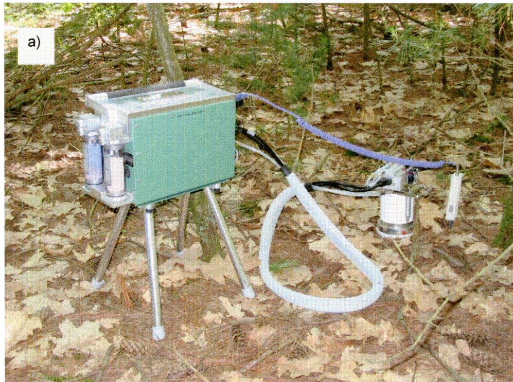
Figure 2.3: a) Above (left) is a photo of the LI-COR 6400 instrument with the 6400-009 soil chamber attachment, used to measure soil respiration during this study. In the photo, the chamber (on the right) is sitting above one of the collars, and the instrument is in the process of measuring soil respiration. Next to the chamber is the soil temperature probe (6400-013), inserted into soil. The green “box” is the console, a computer that controls the instrument. Attached to the left-hand side of the console are soil chemical tubes used to scrub chamber-air of CO 2 . The IRGA analyzer is connected directly to the soil chamber (the rectangular block with plumbing, right on top of the chamber). b) (right) Close-up of an installed summer collar used to support the LI-6400 chamber at each measurement point. Using these collars helped to minimize forest floor disturbance due to frequent sampling.
