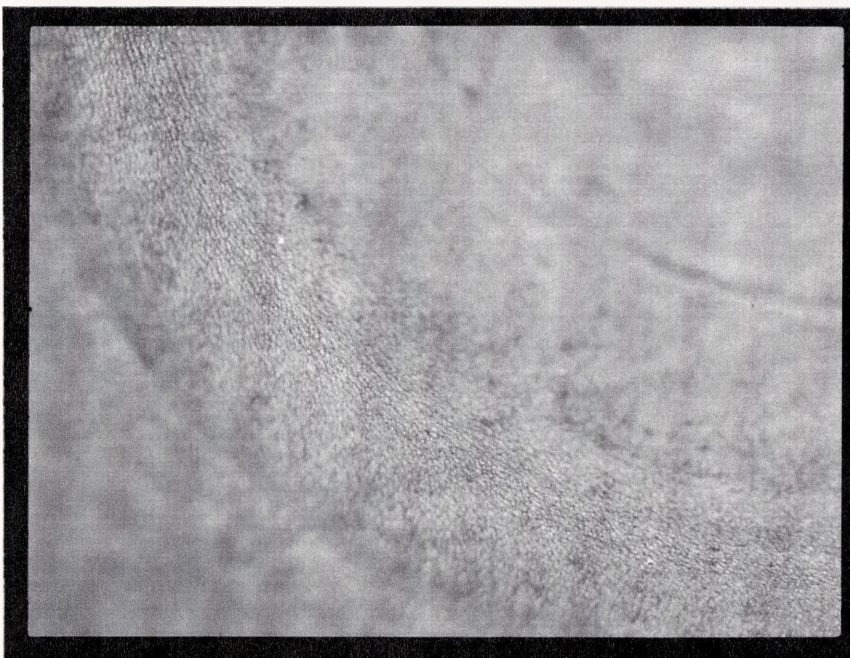
Figure 7.6 Above; photo of a 6.35mm hemispherical shape taken near the top at 200X magnification illustrating elastomer sample surface condition prior to testing. Below; photo of the surface of a 6.35mm hemisphere taken at 192X magnification after two million compression cycles.
