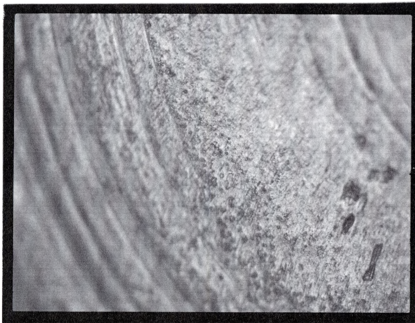
Figure 7.8 Above; Fine scoring of elastomer surface. Photo taken from the flat sheet underside of a 4mm conical featured sample at 160X after 4 million cycles. Note original elastomer surface towards the left and larger cavities to the right. Below; intermediate surface erosion of a 25.4mm hemispherical sample taken at 192X after 2 million cycles.
