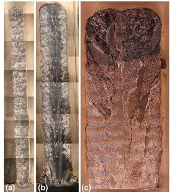
Figure 1.2-3 The complex microstructure of Ti-6Al-4V resulting from rapid melting and cooling from the SLM process [16].
