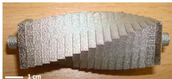
Figure 2-18 The truncheon test part [17]
