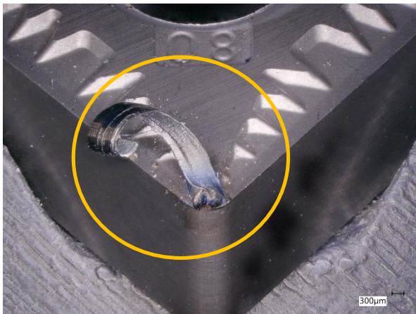
(a) 1 st pass- chip sticking to the rake face
