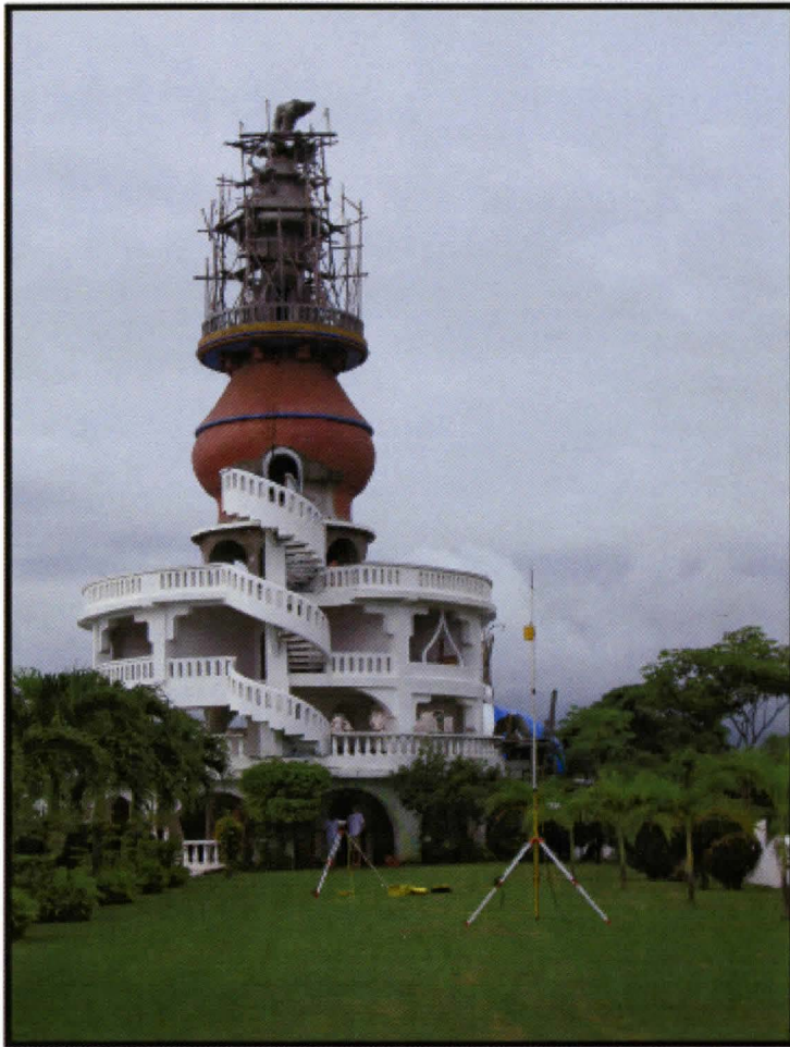
Figure 3.1: An image illustrating the set up of the real-time kinematic GPS unit at Hotel Nosara, Costa Rica. Note the presence of the base station (tripod with the extended pole) and the roving GPS unit (attached to the backpack on the ground).
