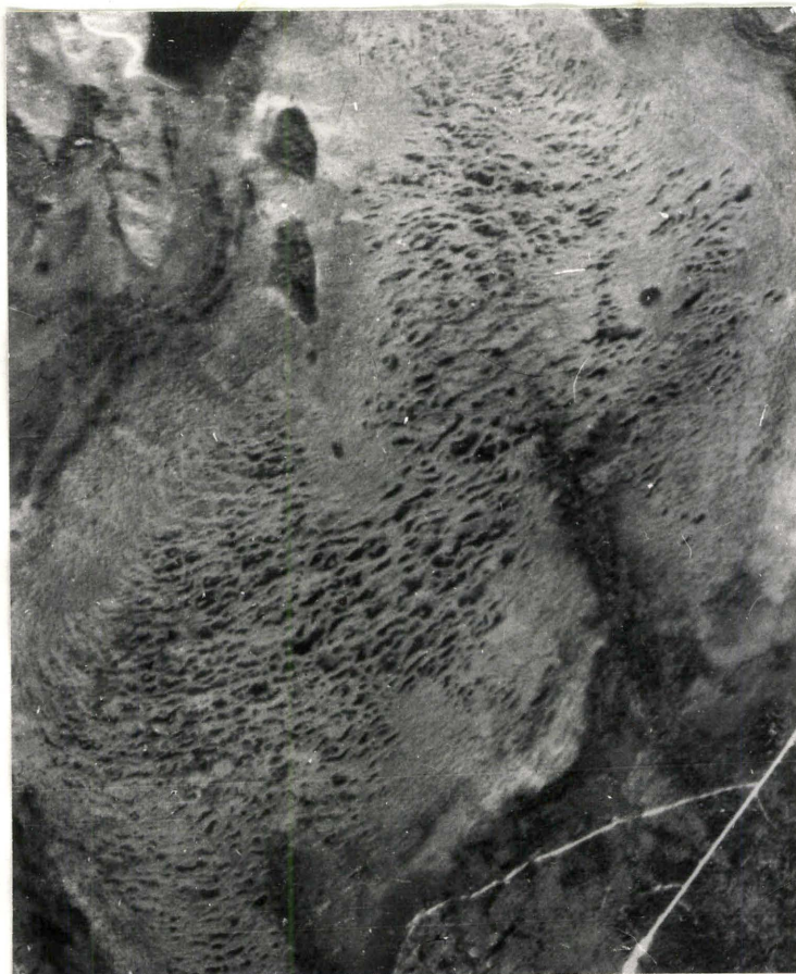
Fig. 127. A high altitude (30,000') vertical airphoto of a raised bog in eastern Canada showing the typical almost concentric ridges of this type of bog.
