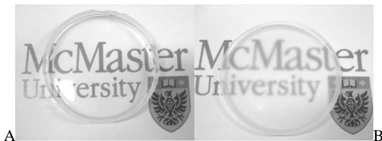
Figure 8.1 Photographs of PEG/silicone elastomers produced using the Huisgen reaction: A: 22 (left), B: 23 (right)
