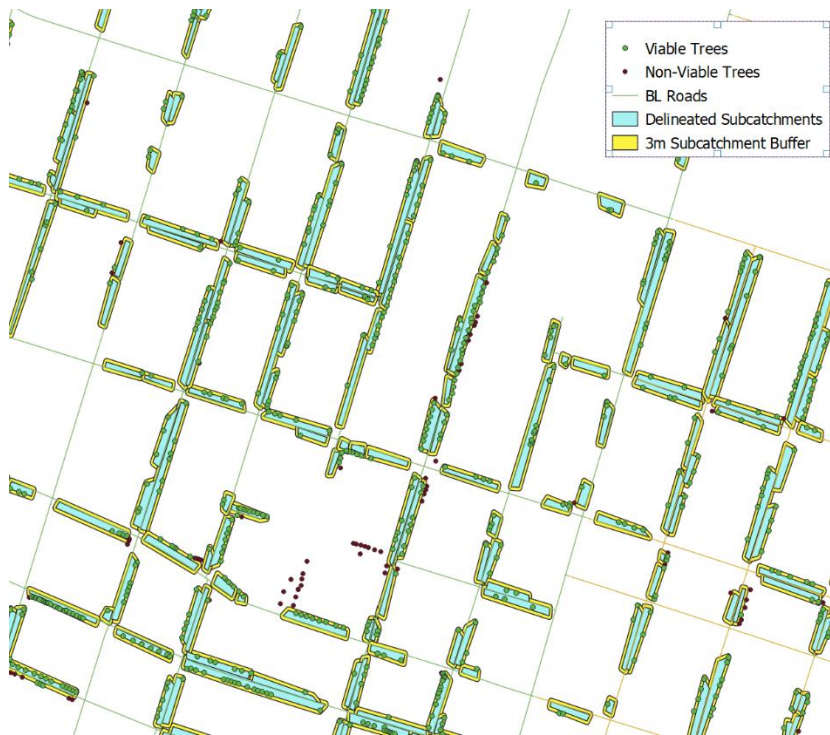
Figure 14: Subcatchments (blue) with 3m buffer (yellow) and viable and non-viable trees. Of 1937 trees within the Study Area, 1762 were deemed to be ideal candidates to accept runoff from adjacent roads. This was determined based on the trees were within 3 metres of the established catchments.
