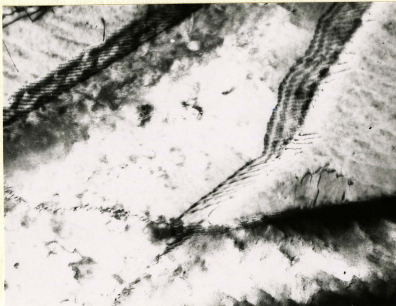
Fig. 29. Widmanstatten plate showing facets formed at 500^{\circ}\text{C} . Note apparent subgrain formed by dislocations emanating from the tip of the plate. X 60,000
