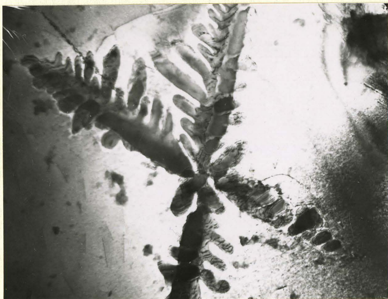
Fig. 17 \gamma precipitate in Cu-Zn-Sn alloy Tempered for 30 min. at 300°C. X 22,000
