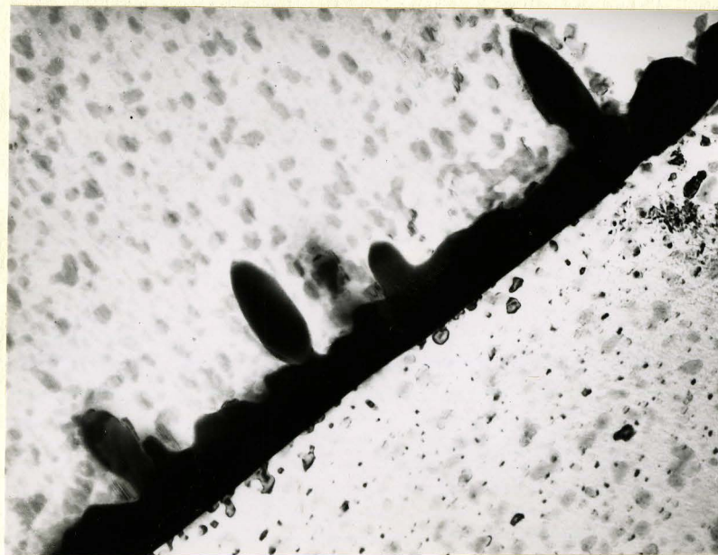
Fig. 19(b) Grain Boundary precipitate in Cu-Zn-Sn alloy Tempered 15 min. at 300°C X 30,000
