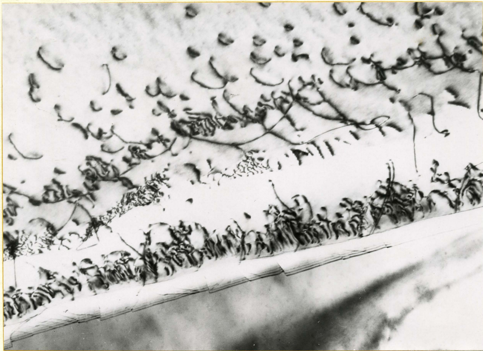
Fig. 25. \alpha - \beta interface formed on tempering at 200°C for 1 hr. showing interface facets and dislocations X 120,000
