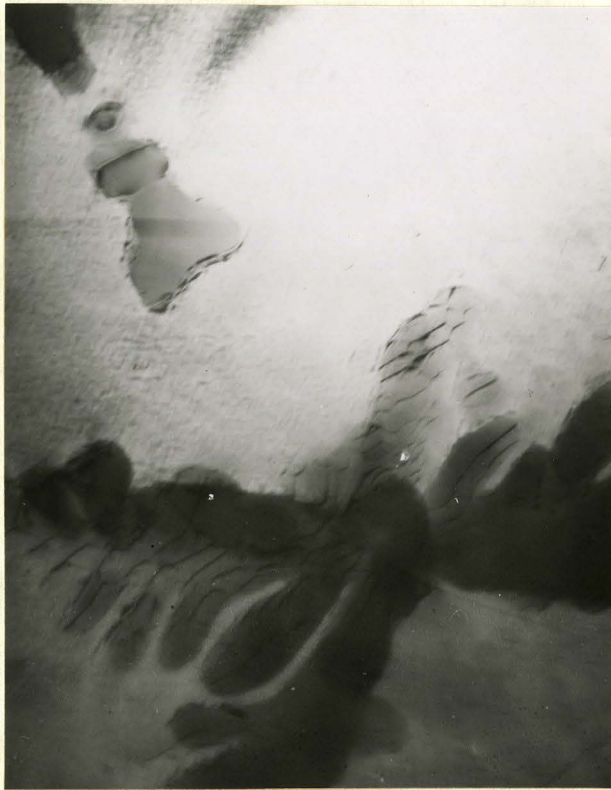
Fig. 16 \gamma precipitate in Cu-Zn-Sn alloy. Tempered for 15 min. at 300°C. X 30,000
