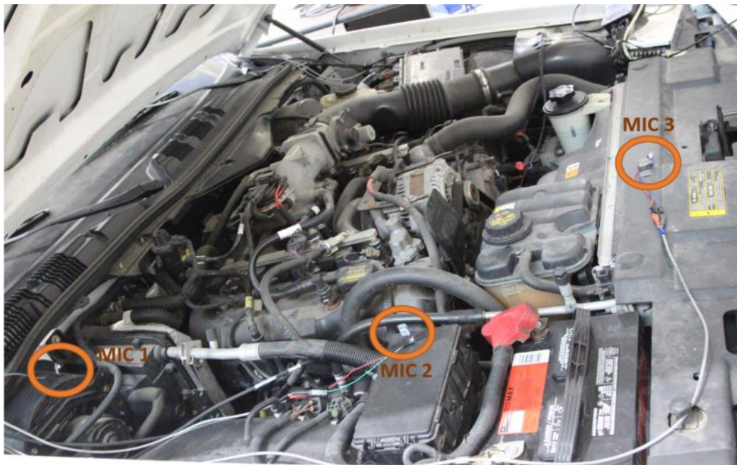
Figure 6.2 Mounting the Microphones
