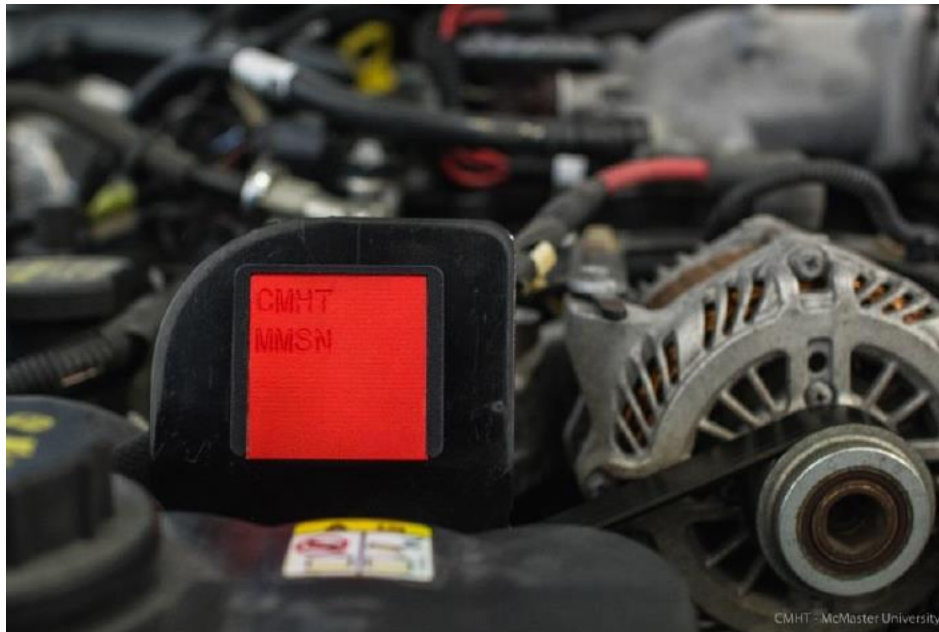
Figure 5.8 FDD Sensor Mounted on the Engine [7]
