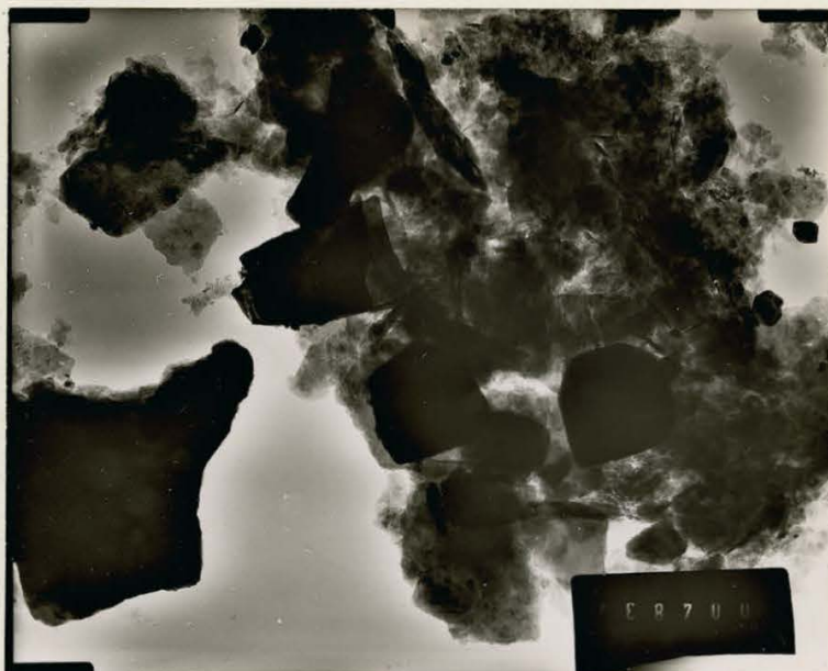
Fig. 90. Illite minerals in the B_{22}^t horizon of the Ancaster series. X 75.000.
