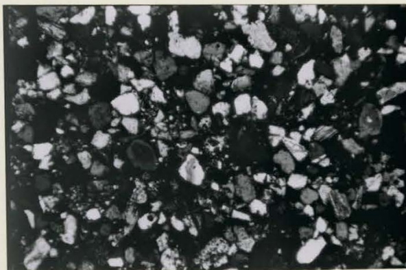
Fig. 54, porous microstructure and compound packing voids in the C_1 horizon of the Port-Cockburn series at 25 inches depth, under normal light. 35X.
