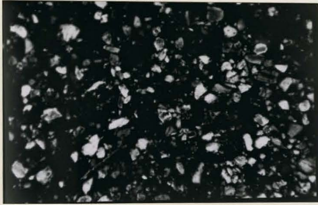
Fig. 72, isotropic plasmic fabric in the A_1 horizon of the Hendrie series at 5 inches depth, under normal light. 35X.
