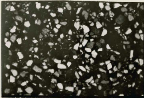
Fig. 64, ortho vughs and porous microstructure in the B_{2t} horizon of the Alliston series at 30 inches depth, under normal light. 35X.
