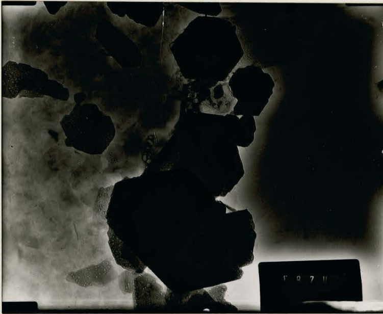
Fig. 89. Kaolinite clay minerals with well crystallized structure in the B 22 t horizon of the Huron series. X 80.000.
