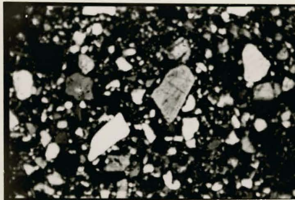
Fig. 74, skel-insepic plasmic fabric in the C_1g horizon of the Hendrie series at 30 inches depth, under normal light. 35X.
