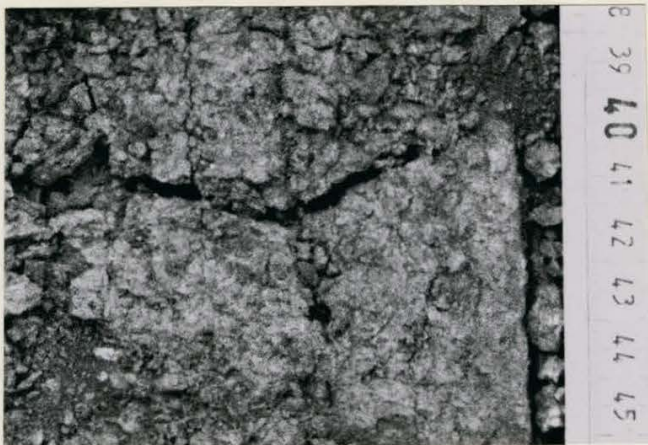
Fig. 27, medium angular blocky structure in the B 22 tg horizon of the Winona series.
