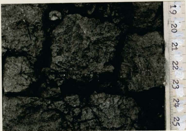
Fig. 15, coarse angular blocky structure in the B_2^t horizon of the Ancaster series.
