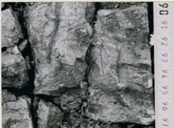
Fig. 22, coarse angular blocky structure in the Cg horizon of the Vineland series.
