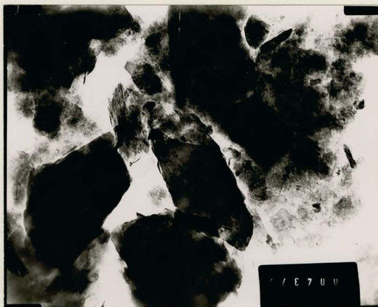
Fig. 87. Kaolinite clay minerals with poor crystallized structure in the B_{22}^t horizon of the Guelph series. X 80.000.
