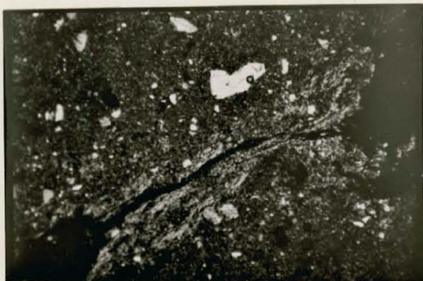
Fig. 30, bi-masepic plasmic fabric and craze planar voids in the B 22 tg horizon of the Winona series at 15 inches depth, under normal light. 35X.
