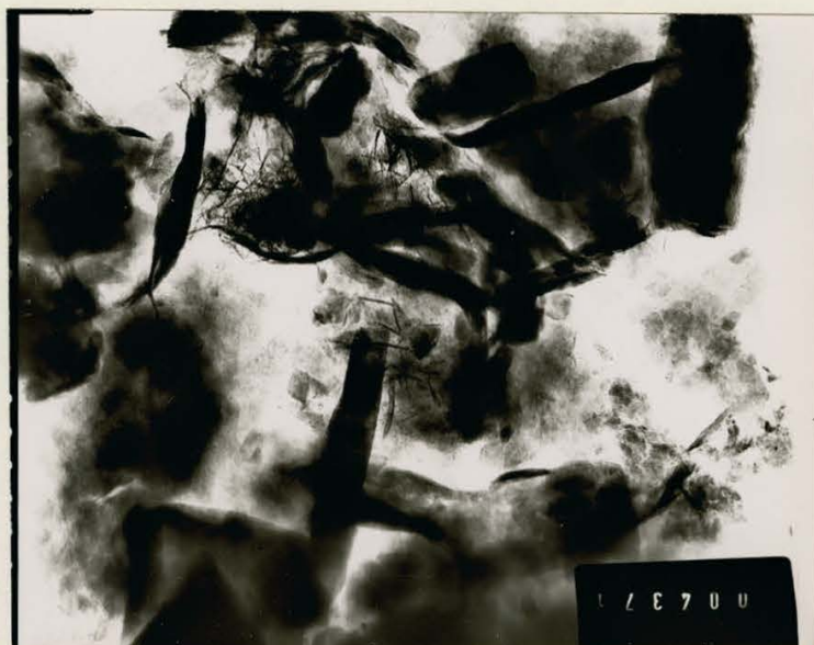
Fig. 91. Mixed layer mica-montmorillonite clay minerals partially ordered structure in the B_{22}^t horizon of the Winona series. X 90.000.
