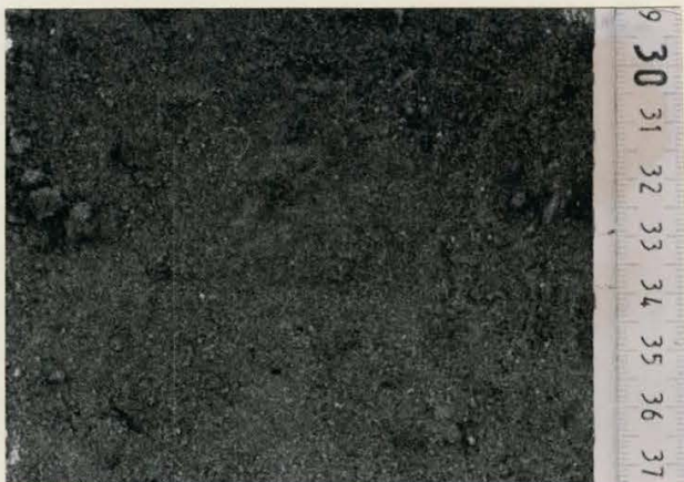
Fig. 16, fine granular structure in the IIC_1 horizon of the Ancaster series.
