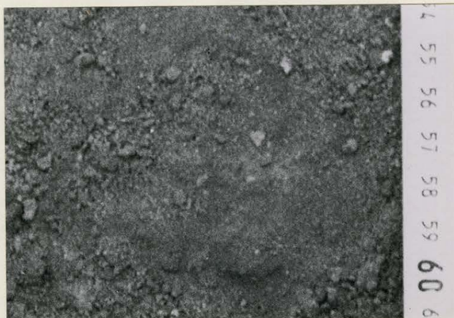
Fig. 51, fine granular structure mixed with small and medium gravels (25 %) in the C_1 horizon of the Port-Cockburn series.
