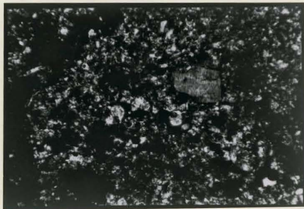
Fig. 25, regular nodule with rock fabric (lithorelict) and an ortho vugh in the Cg horizon of the Vineland series at 40 inches depth, under normal light. 35X.
