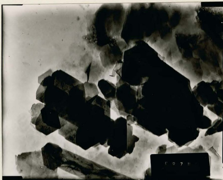
Fig. 86. Kaolinite clay minerals with well crystallized structure in the B_{22}^t horizon of the Haldimand series. X 80.000.
