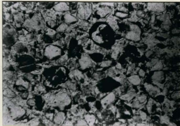
Fig. 73, skelsepic plasmic fabric and simple packing voids in the B_{22} horizon of the Hendrie series at 10 inches depth under normal light. 35X.
