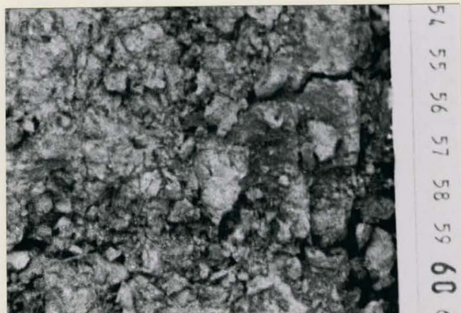
Fig. 28, fine angular blocky structure in the Cg horizon of the Winona series.
