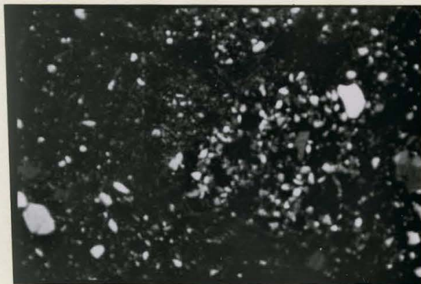
Fig. 13, silasepic plasmic fabric in the IIC x horizon of the Guelph series at 35 inches depth, under normal light. 35X.
