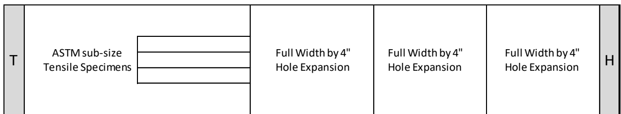
Figure 3.1. Sample shearing for hole expansion testing and tensile testing
