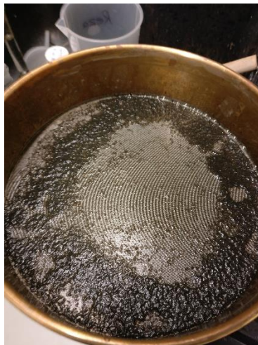
Figure 4.2: 0.3 mm screen used for pretreatment including the solids that were separated from 8L of centrate.
