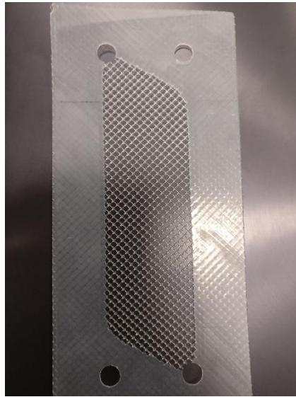
Figure 4.1: 0.8 mm thick sheet flow spacer constructed from ethylene-vinyl acetate used to separate membranes and create a flow path.
