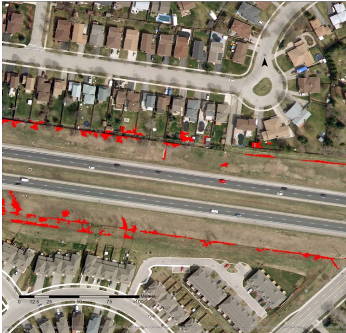
Figure 9.13: Sample of orthophoto over Hwy 85 showing Phragmites classified in red. Although some error is expected and some Phragmites had been accurately classified, the unique configuration of the built-up area led to numerous errors of commission.
