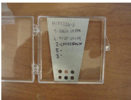
Figure 3.5 Samples on the special holder for STXM characterization. The TEM grids are on the holes for the experiments.
