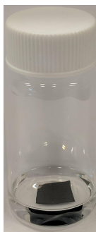
FIGURE 5.6: Photograph of the PF-N 3 -SWNT functionalization process. A 1 cm 2 PF-N 3 -SWNT thin film is soaked in a solution of strained cyclooctyne.
