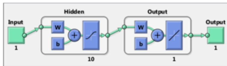
Figure 6-16: Fitting Tool Architecture
